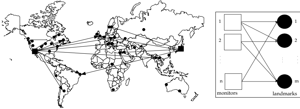
Fig. 2. Distributed Top-k query processing in the context of Internet Traffic Monitoring: The illustration on the left presents two monitors (squares) that ping a number of landmarks (dots). The collected data is utilized to infer topological properties about the Internet. A Top-k query is to find the k landmarks (regions) with the highest score in some specified metric (loss, delay, etc). The figure on the right depicts the bipartite graph abstraction of this scenario.
