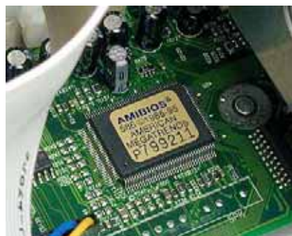
Figure 5.3: BIOS uses Flash memory, a type of ROM.
